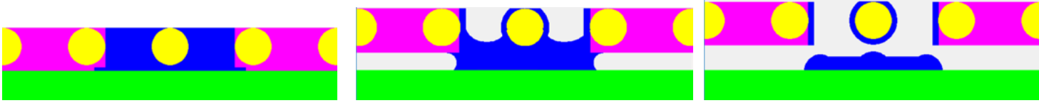
Figure 8-4 A high roughness (Rz) allows ink to get under the edge of the stencil, giving ragged dot gain ("positive sawtoothing").
